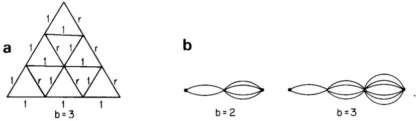
Fig. 3. (a) The case where the left-leaned resistors have resistance  $r$  ( $0 < r < 1$ ). (b) Reductions into unit resistor networks for the case  $r = 0$ .
