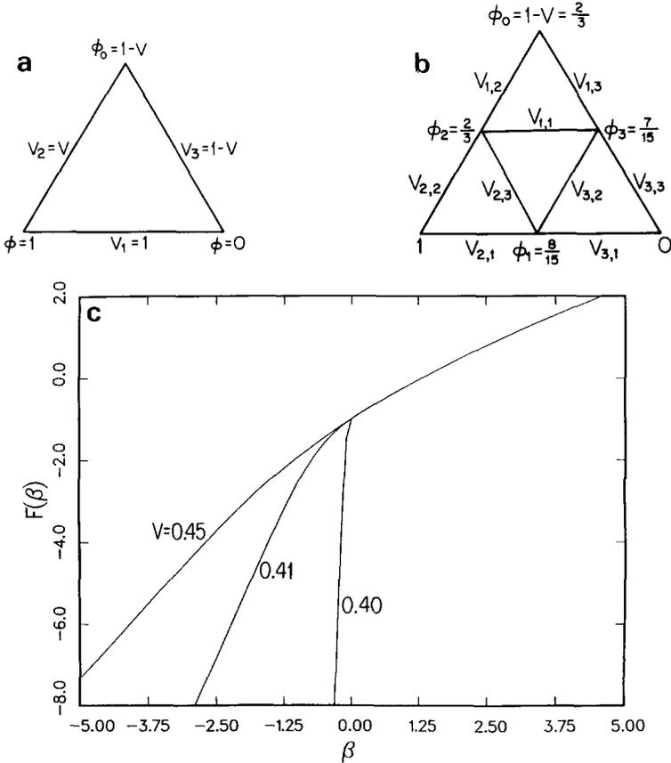
Fig. 1. (a) Notation for potentials  $\phi$  and voltage drops  $V_j [j=1-3]$  for the basic triangle from which are generated the hierarchy of Sierpinski gasket fractal resistor networks. Note that  $V$  is the only tunable parameter.
