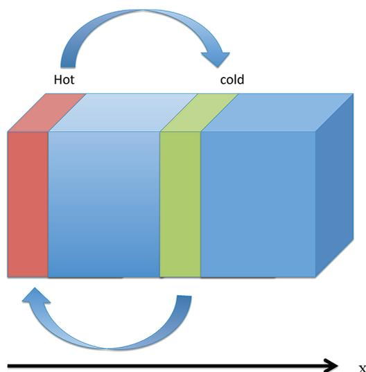
**Figure 2.** To use the MP algorithm to calculate the thermal conductivity, the simulation box was divided into  $N_{\text{slab}} = 12$  slabs along the  $x$  direction. The first and central slabs were then chosen as the hot and cold regions, respectively, for swapping molecules.
