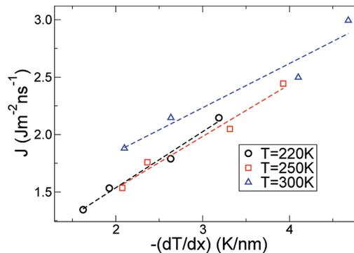
**Figure 3.** Heat flux  $J$  for three different temperatures as a function of the temperature gradient  $-(\langle \partial T / \partial x \rangle)$ . Dashed lines are linear fits through the data, suggesting a linear regime at these flux values.
