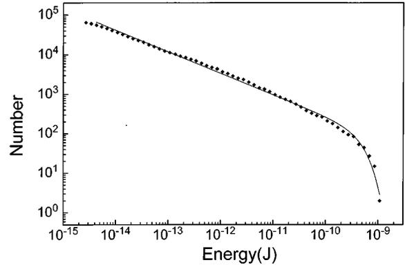
FIG. 5. Experimental data for the distribution of signal energies (diamonds) and the best fit curve [of the power-law type, with the correction factor of the form (27)]. The critical exponent  $\epsilon=1.56$  describes the scaling region.
