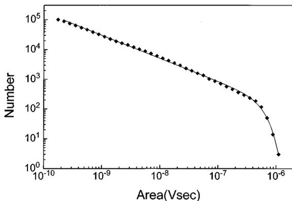
FIG. 4. Experimental data for the distribution of signal areas (diamonds) and the best fit curve [of the power-law type, with the correction factor of the form (22)]. The critical exponent  $\tau=1.77$  describes the scaling region.
