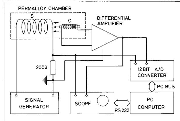
FIG. 1. A schematic depiction of the setup used in the experimental course of this work. The ballast resistor of  $200\ \Omega$  has been used to reduce the influence of Barkhausen noise on the current which flows through the driving solenoid  $S$ .
