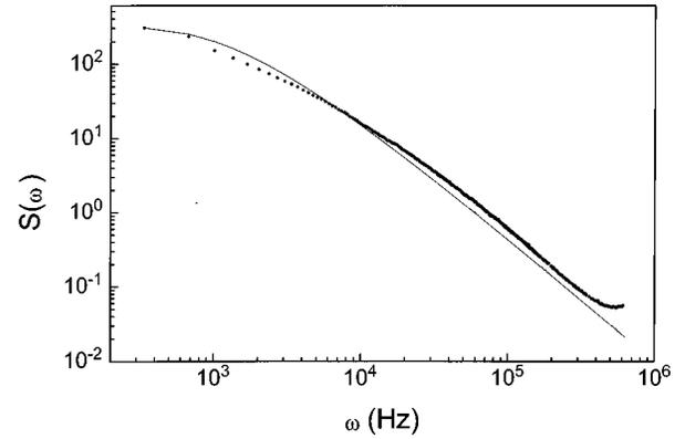
FIG. 9. Power spectrum  $S(\omega)$  (in arbitrary units) of the observed BN signals. The set of points (dots) is calculated via the FFT method and represent experimental findings, whereas the solid curve represents numerical evaluation of (38).
