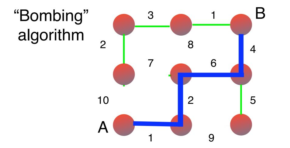
Optimal path between A and B is the Min-Max path  $\equiv$  path with the lowest maximal weight along the path.
